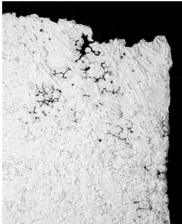
Figure 6. Hydrogen embrittlement damage in a chain link. 100x.
