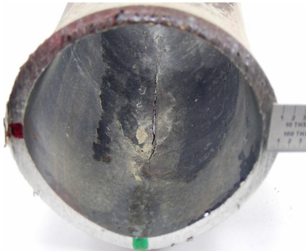
Figure 3. Stress-corrosion cracking at the bottom of a reheat tube bend.
