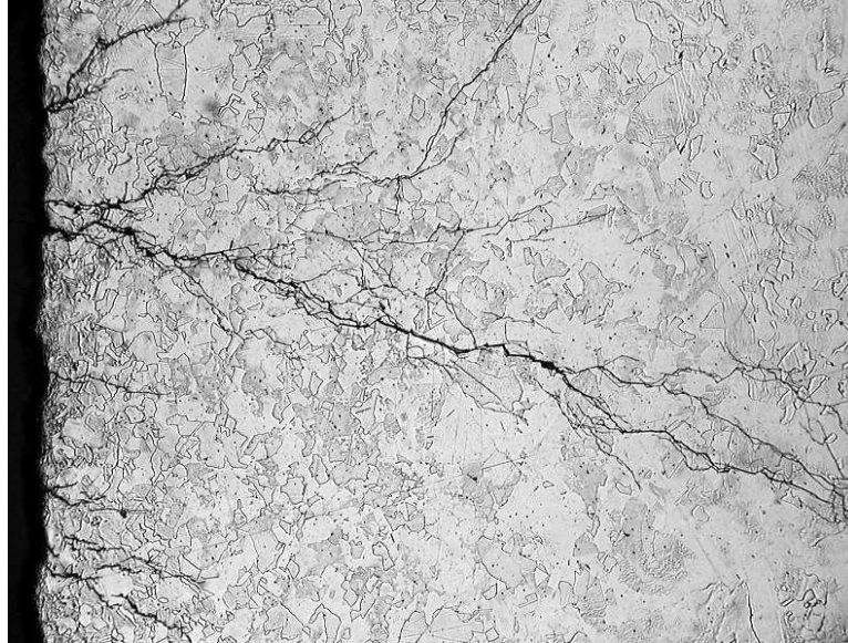
Figure 2. Severe branching of transgranular cracks in 304H stainless steel flange. 50x.
